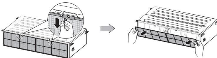
2. Clean the Air filter with a vacuum cleaner or soft brush. If dust is too heavy, then rinse it with running water and dry it in a ventilated area.
