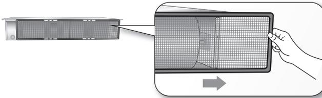
2. Clean the Air filter with a vacuum cleaner or soft brush. If dust is too heavy, then rinse it with running water and dry it in a ventilated area.
