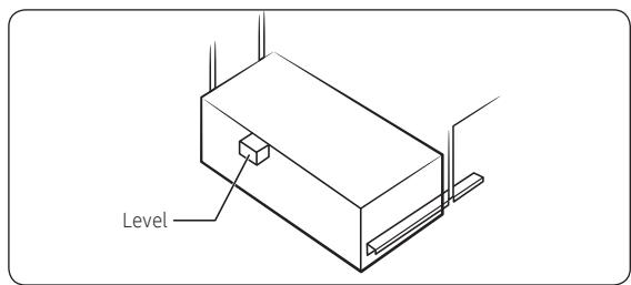
7 Adjust the unit to the appropriate position, taking into account the installation area for the front panel.
